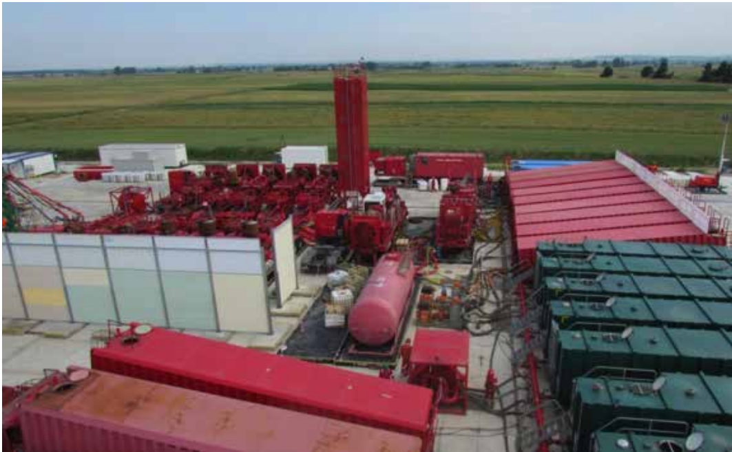
Figure 4: Hydraulic fracturing installation showing storage tanks, bunded fracturing fluid product containers and a vertical sand tower
